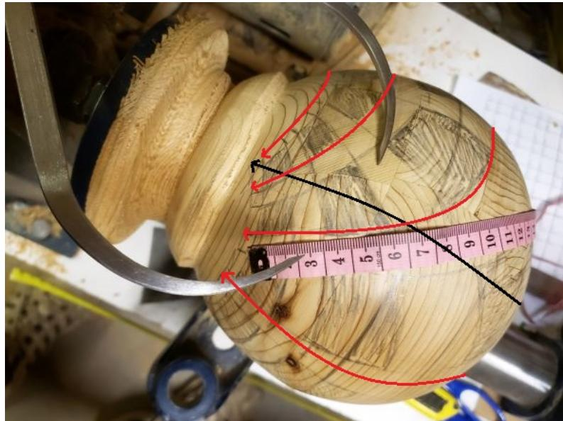
The arc lengths we found in the "Build Plan" section are shown in red in the picture above. To check our measurements, it would be good to also know the length of the black line in this picture. This will be the longest length around the globe. It will be one quarter distance to the red line that goes from the bottom of the well all the way around the sphere. The four max points, and the four well points will give a solid starting point for locating the cutouts.
